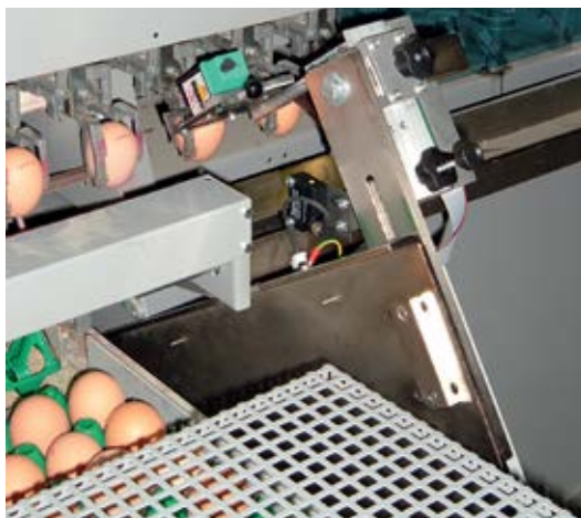
A print half way onto blunt end of the egg in a farm packer. The printers are equipped with a start sensor. If the sensor is dirty, misprints will occur, and eggs will be missed totally or incorrectly printed.
