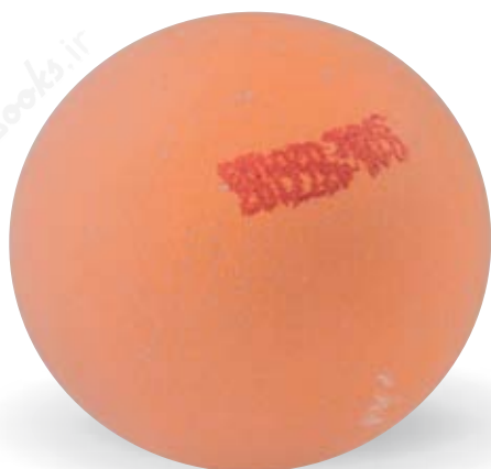
Smudged print caused by unsuitable ink or a dirty shell.
