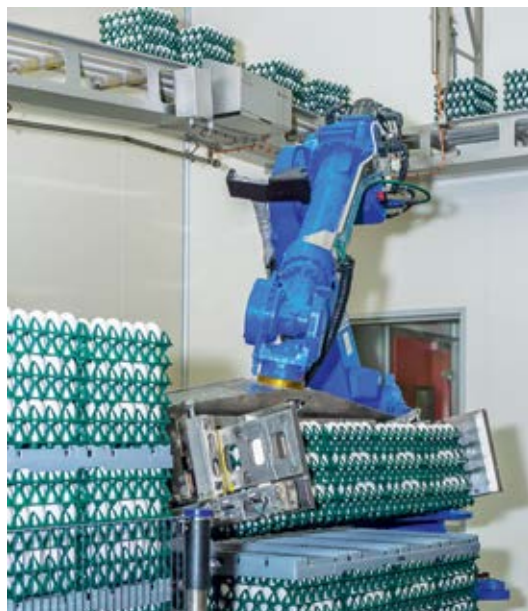
The loading robot takes eggs in layers of six trays from the pallets and puts them on the conveyor.
