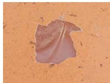
The eggshell usually remains intact after you break them off (unlike with pinholes or implosions).
