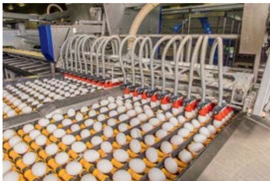
Once removed from the stack and trays, the eggs are put on the belt, which transports them to the dirt detection unit.
