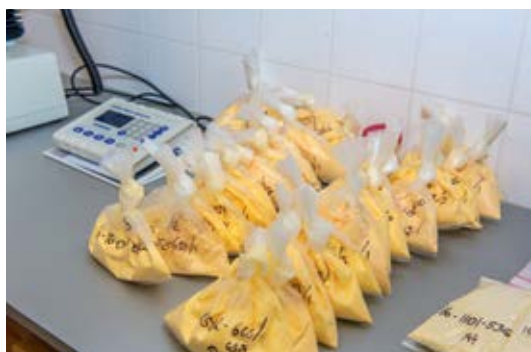
Besides inspection on delivery, egg products are checked before shipping. These include tests for pH, moisture, fat, protein, lactic and butyric acid content. The bacteriologic composition is also assessed. Sometimes, there are tests for the albumen foaming ability, and salt or ash content.
