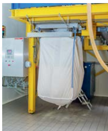
Egg powder is put in Big Bags (left), or in 25-kg plastic bags, which are then put in cardboard boxes (bag-in-box).
