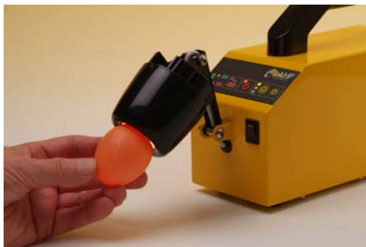
Cracks might be due to a decreased shell strength and can be detected by candling.
