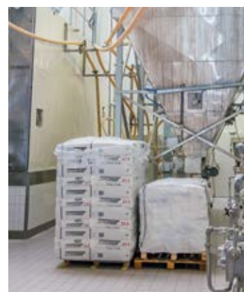
Egg powder is put in Big Bags (left), or in 25-kg plastic bags, which are then put in cardboard boxes (bag-in-box).
