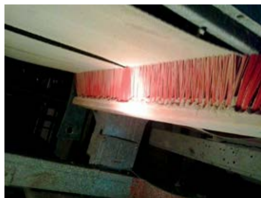
Fitting a brush under the egg belt will continuously clean the belt while it runs. It is a simple and very effective solution.
