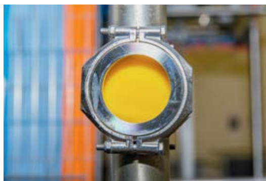
Viewing points in the pipework allow you to see which product is pumping through, whole egg, yolk, or egg white.
