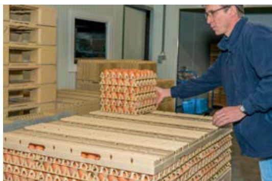
Eggs are usually delivered to packing stations in stacks of plastic trays, with six on top of each other per layer. There is a dividing plate before the next layer. The operation repeats until there are five layers on the pallet.
